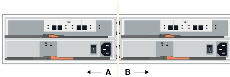
2. Connect the cables to A-side IOM12 ports three and four from the new shelf to previous last shelf IOM12 ports one and two.
